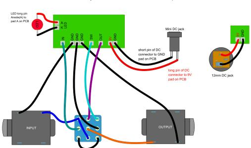
2. Radial jacks - WIRING with off board LED - L+ pad
