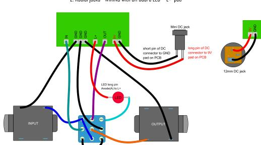
3. Axial jacks - WIRING with on board LED pads, SW pad
